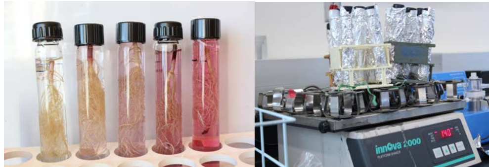
Figure A-2: Photos from the sorption experiment (Experiment 5). On the left are the capped roots from ascending concentration order from left to right: 0.0 mg/L, 2.0 mg/L, 5.0 mg/L, 10.0 mg/L and 15.0 mg/L. The right photo shows the test tubes on the shaker.
