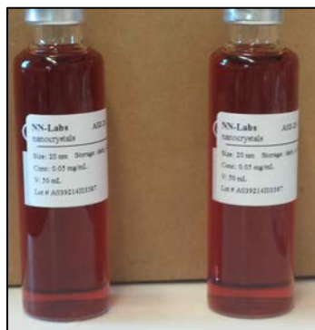
Figure 3-3: 50 mL containers of 20 nm Au NPs at 0.05 mg/mL stabilized with citrate and dispersed in H 2 O
