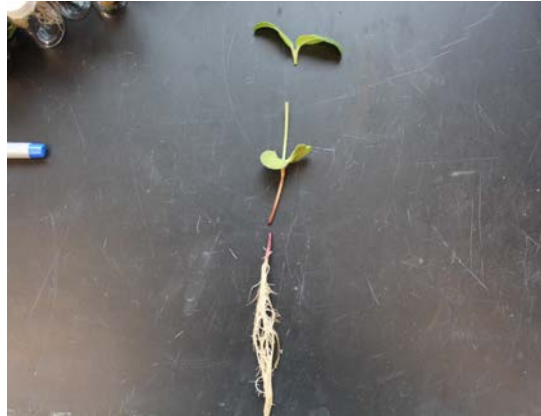
FigureA-1: A photo of the separate part of the sunflower that were tested for biomass and ICP-MS of the roots stems and leaves.
